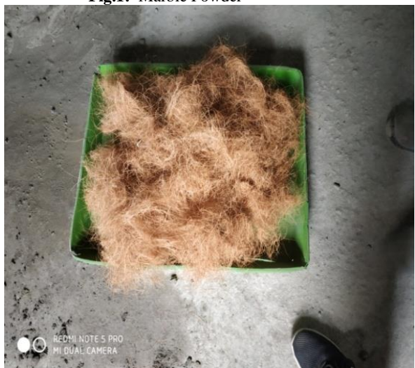
Fig. 2: Coconut Coir Fibers
